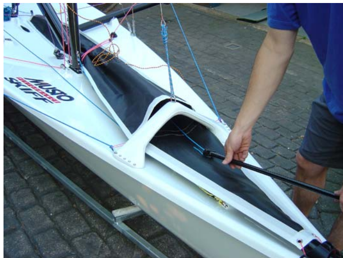
48. Pull the extension out of the chute
