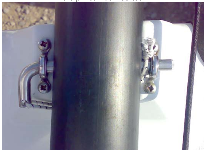
13. With the elastic between the wing and the deck eye the elastic can never get knocked off and you won't lose any pins. The folded ends of the pins should be away from the cockpit so that the mainsheet doesn't get caught on the pin.
