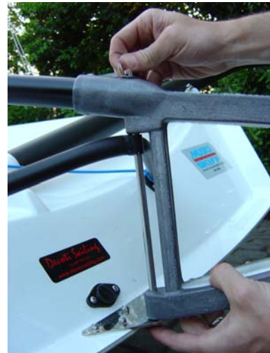
64. Insert the split ring at the top to hold the pin in place. Once on the stock it can be left on the boat permanently.
