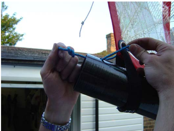
76. Back through the hole in the boom.
