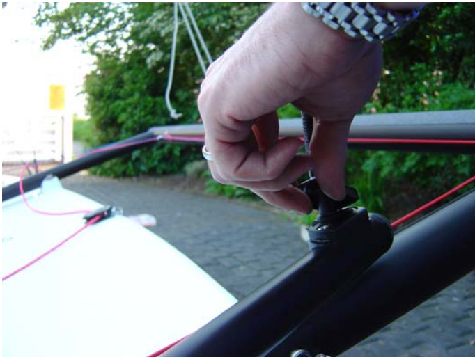
65. Clip the tiller extension onto the tiller.
