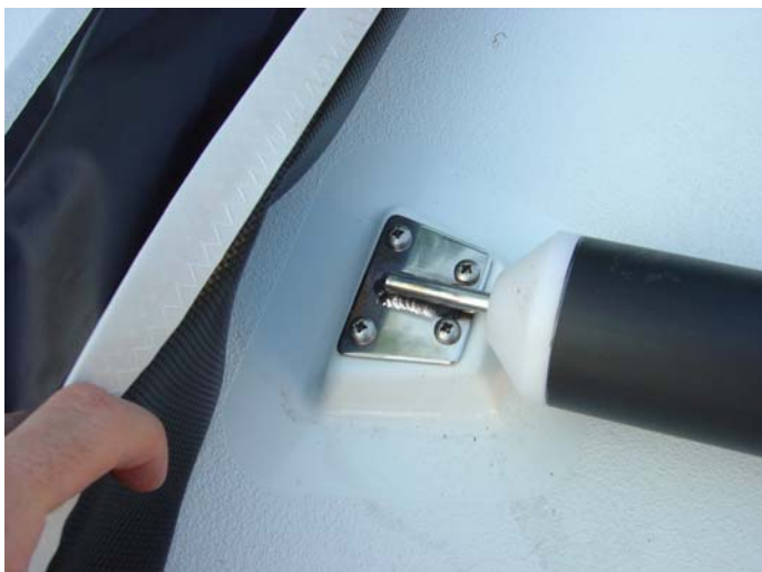
10. Fitting the wings is simple; make sure you align the white end fittings with the male fitting on the deck.
