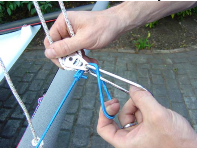
25. Take the loop around the trapeze ring
