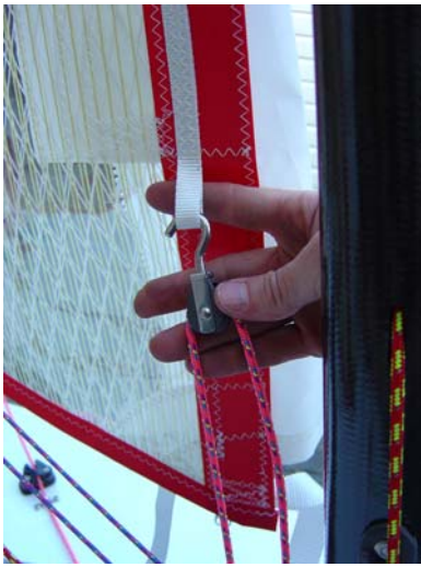
81. Hook the port downhaul block to the port loop
