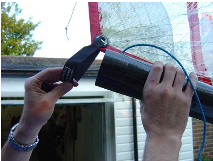
74. Post the clew strap over the end of the boom. Musto Performance Skiff – Rigging Guide (v0.4)
